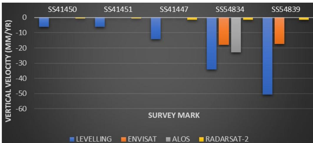
Figure 16: Vertical (up-down) velocities (mm/yr) determined by differential levelling and each InSAR mission.
