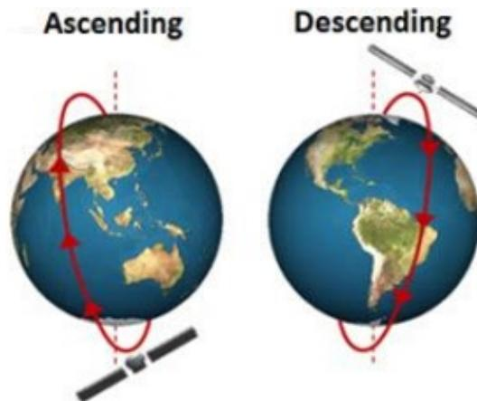
Figure 4: Diagrammatic representation of an ascending and a descending orbital pass (Garthwaite and Fuhrmann, 2020).
