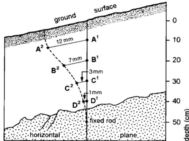
A<sup>1</sup>B<sup>1</sup>C<sup>1</sup>D<sup>1</sup> Initial position of rods
