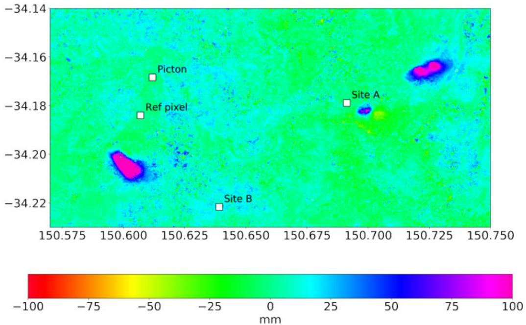
Figure 18: Areas of subsidence in the NSW Southern Coalfield determined using the Sentinel-1 mission. The Tahmoor mine is located in the south-western corner of the image (GA, 2017).
