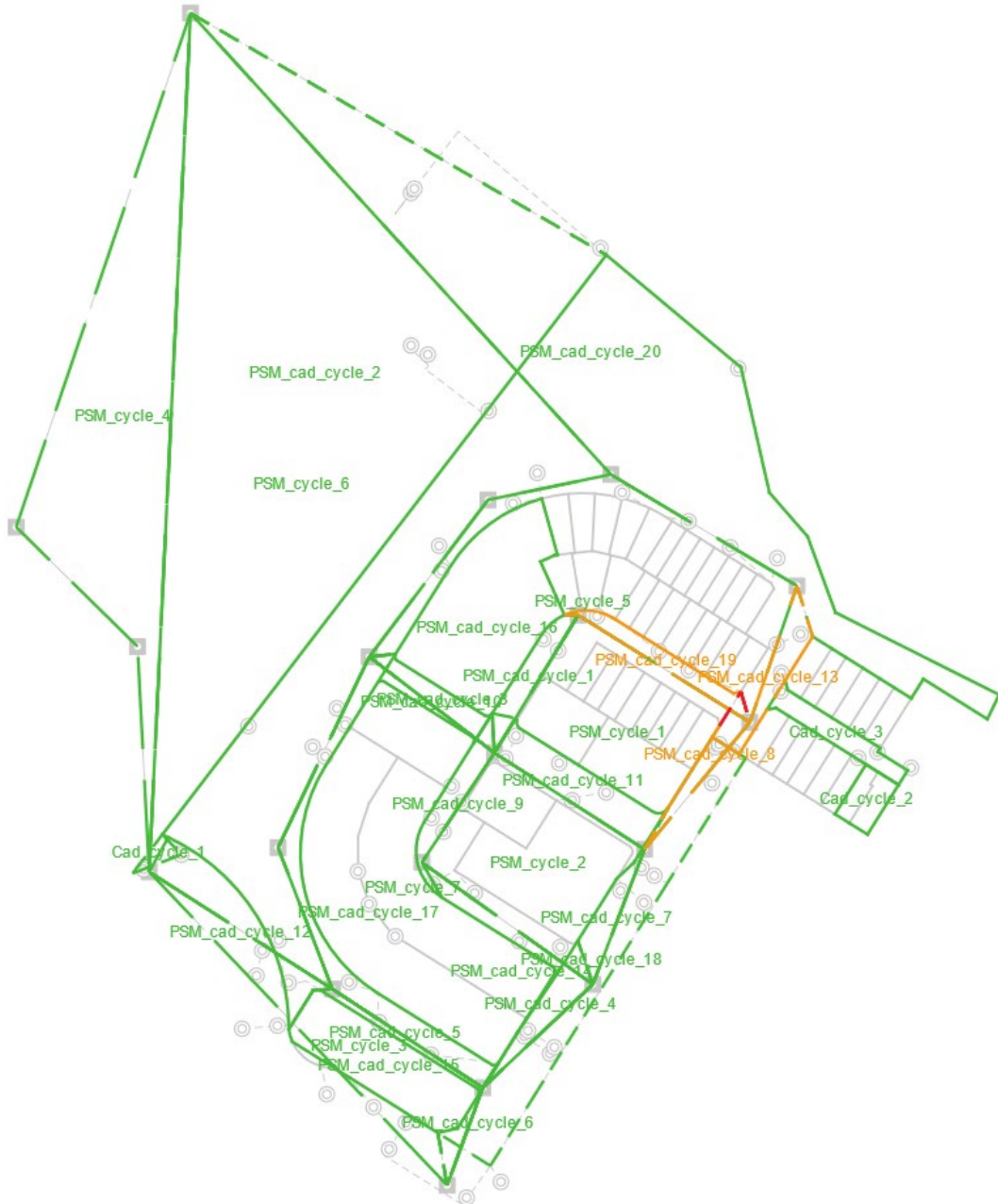
Figure 8: MIR extracted cycles health diagram example, indicating problematic cycles (orange = suspect, red = possible error).
