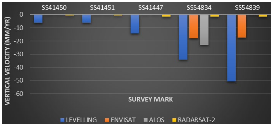
Figure 16: Vertical (up-down) velocities (mm/yr) determined by differential levelling and each InSAR mission.
