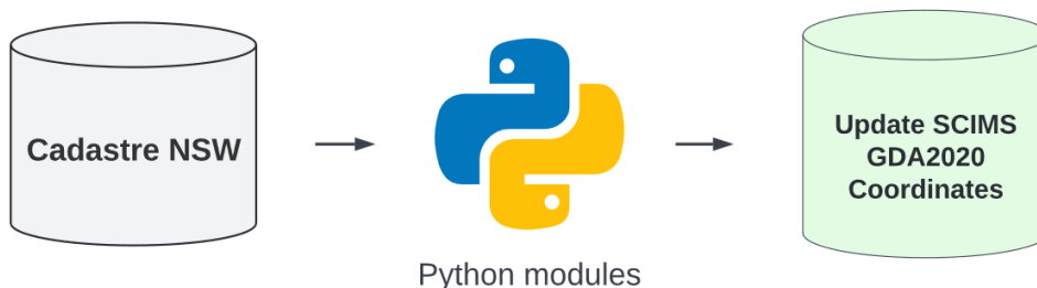
Figure 3: Concept of harvesting LandXML control data to update SCIMS.
