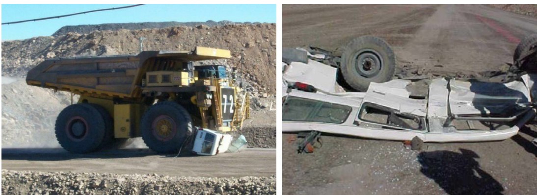
Figure 2: (a) Dump truck impacting on a light vehicle and (b) the aftermath (Mining Mayhem, 2010).
