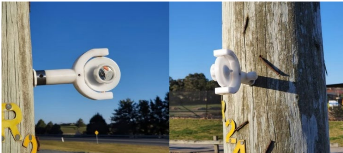
Figure 5: Spigot reflectors mounted to a power pole. The spigot screws into a ‘wall plug’ that rests firmly inside a hold drilled into the pole. The reflector can turn freely on two axes in any direction, allowing measurements of the same point to be taken from both sides.
