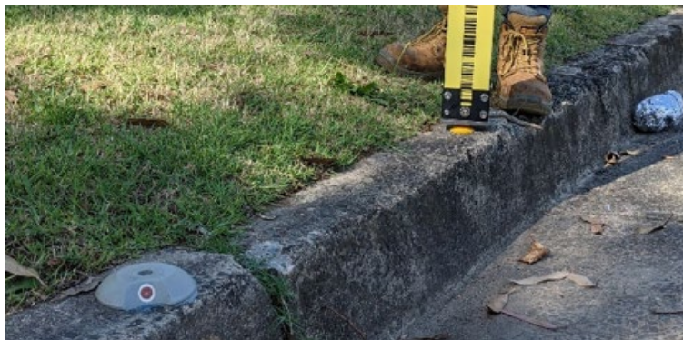
Figure 13: Close proximity of the starting benchmark reflector for OPL (left) and the starting nail for digital levelling below the 2 m invar staff (right).
