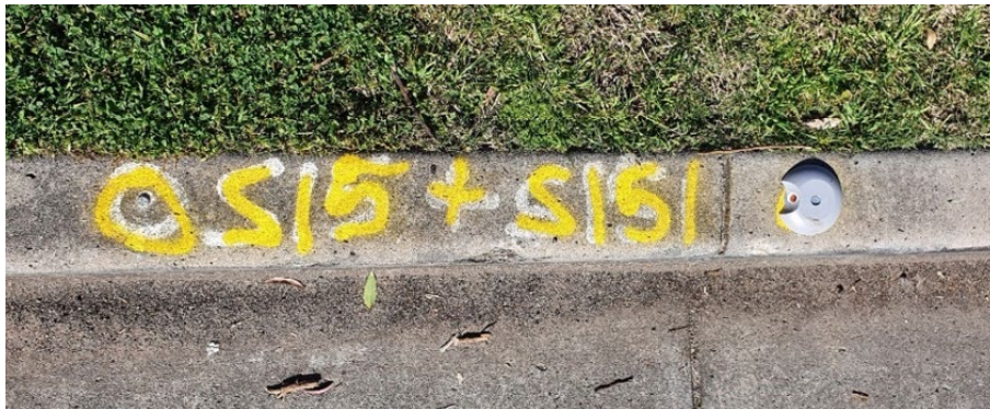
Figure 9: Levelling nail (left) adjacent to a ground target (right) on the kerb, in close enough proximity to check if movements between the marks are consistent.
